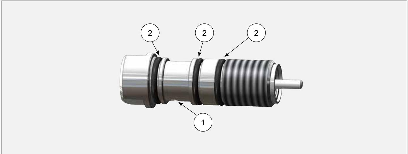
**REAR CARTRIDGE ASSEMBLY 80262-01 (NON-ADJUSTABLE FLUID CONTROL)**
