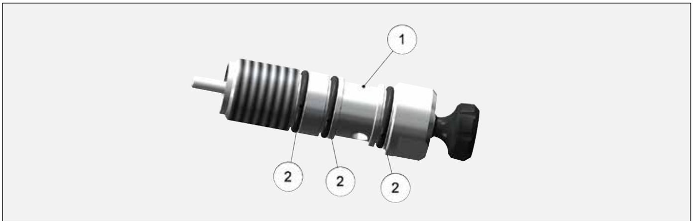
**REAR CARTRIDGE ASSEMBLY 80262-00 (ADJUSTABLE FLUID CONTROL)**
