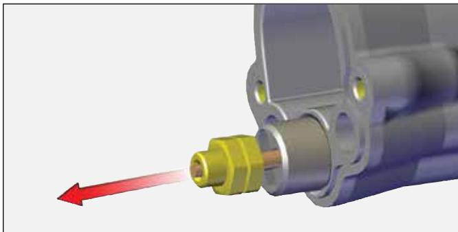
4. Remove jam nuts using 10mm wrench.
