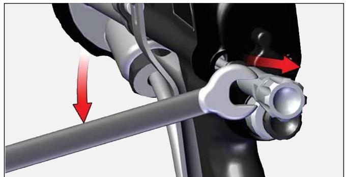
3. Remove rear cover and cartridge with 15mm wrench.
