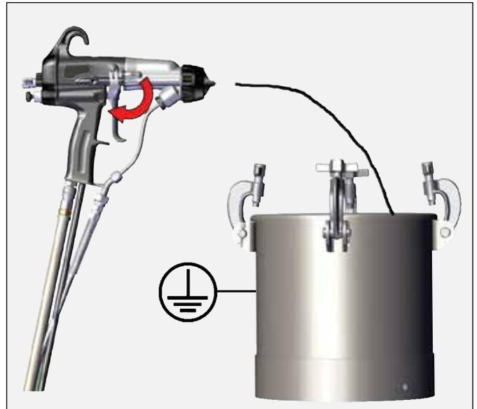
4. Load next color, solvent flush and/or remove applicator from installation as required.
