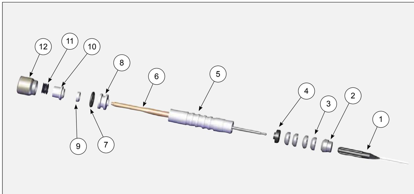
**RFXi 65kV NEEDLE SHAFT 80263-65**
