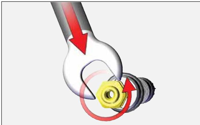
5. Remove all parts, clean with non-polar solvent. Inspect for any discolored areas. Replace parts as required.
