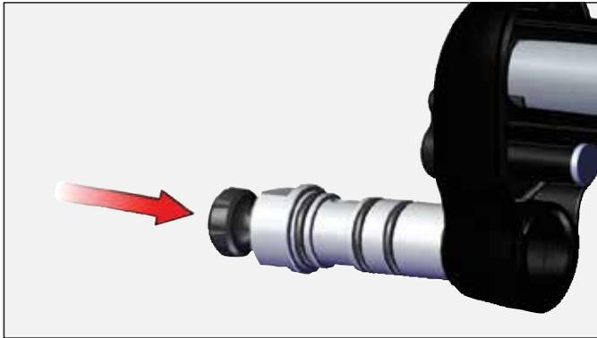
7. Install gasket and re-connect motor connector to handle harness connector.
