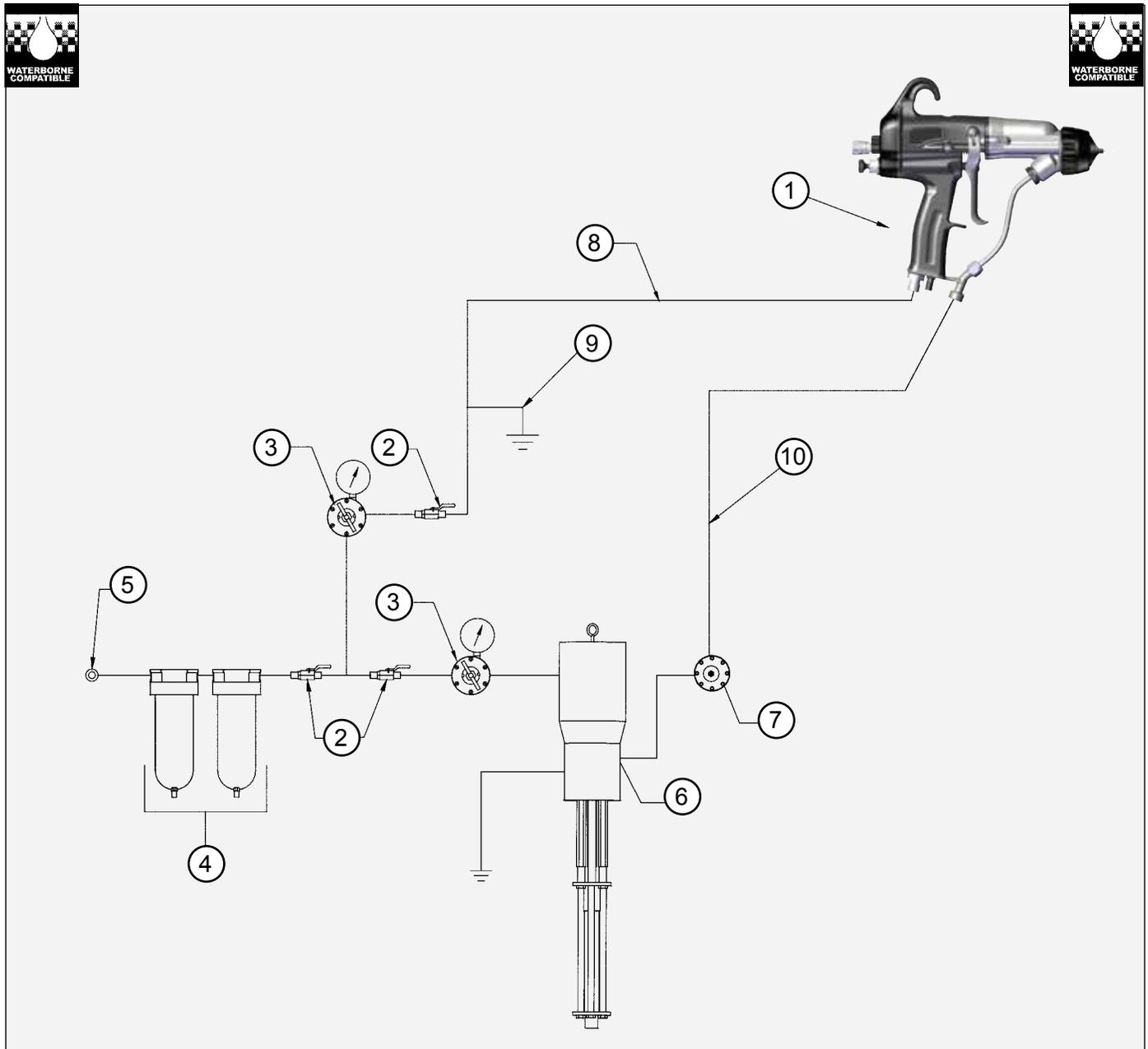
Figure 2: Ransflex Installation for Waterbase Materials
