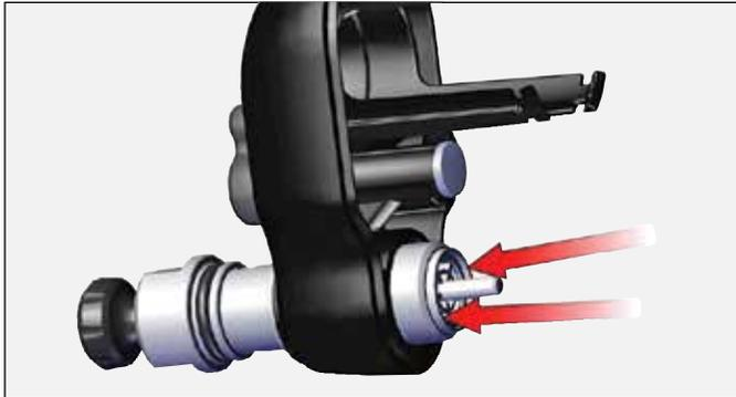
3. Install cartridge then o-ring (if removed).
