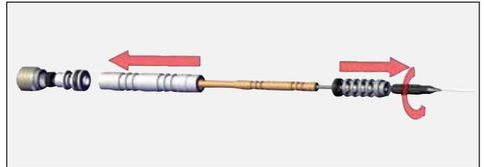
6. Prior to installation apply dielectric grease inside packing tube, completely full.
