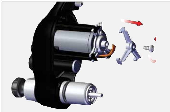
3. Remove motor assembly by pulling out on 3 arms, pull motor out.
