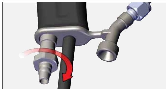
3. Remove bracket, gasket and o-ring.
