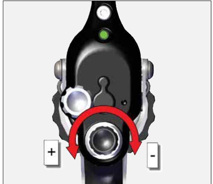
15. Adjust compensation valve with small driver.
