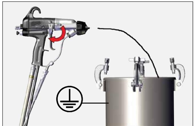
4. Release trigger stop material flow.
