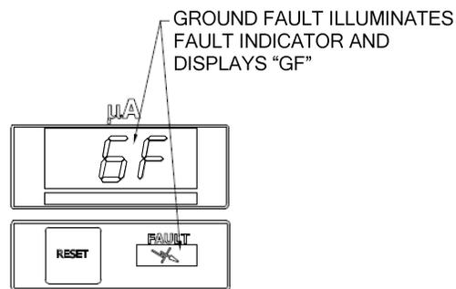
Figure 12: Ground Fault Display
