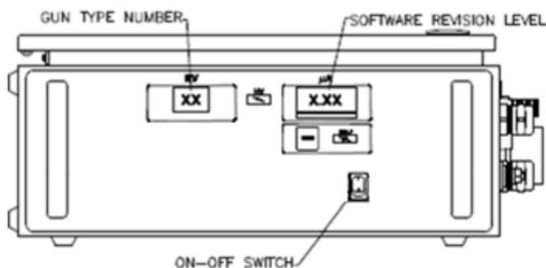
Figure 8: Controller Start-Up Display
