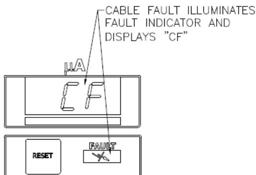
Figure 11: Cable Fault Display
