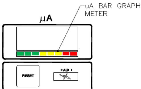
Figure 9:  $\mu$ A Bar Graph Meter Display
