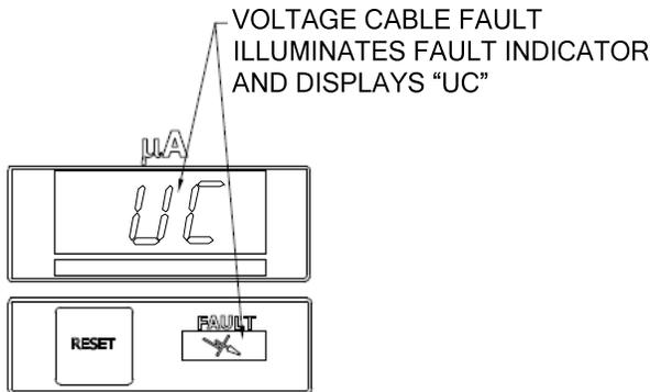
Figure 14: Voltage Cable Fault Display
