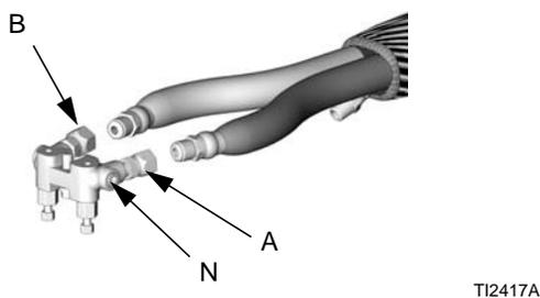
4. Apply thread sealant to plugs (Z), elbows (AA), and male threads of swivels (R). Install elbows (V) in optional inlets (N), facing down. Install swivels (A, B) in elbows. Be sure to install A swivel (smaller) in A side. Install plugs (Z) where swivels had been. Torque all parts to 235-245 in-lb (26.6-27.7 N•m).
