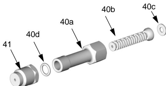
**6.** Reassemble static mixer assembly (40a-e).
