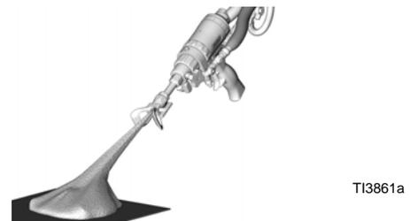
**15.** Apply layer of lubricant over front of gun and lock ring, or use gun cover to prevent overspray buildup and ease disassembly.
