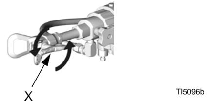
**14.** Test spray onto cardboard. Adjust pressure, temperature, or orifice size to get desired results. If applying materials that are greater than 1:1 ratio, follow the instructions for increasing orifice size, see **Drilling of Mix Modules**, page 15.
