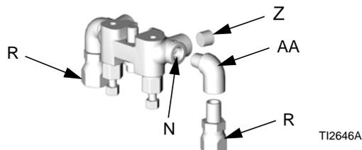
5. Connect appropriate hoses to A and B swivels.
