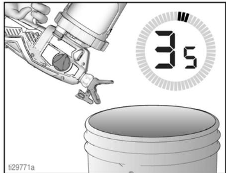
9. Turn Prime Pump/Spray knob forward to spray position. Remove cup assembly and pour any remaining Pump Armour back into Pump Armor bottle. Replace child-resistant cap and tighten securely for storage.
