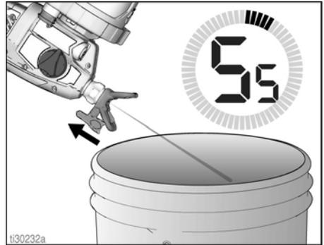
13. If second spray tip was used, remove cleaned spray tip from spray tip guard and install second spray tip. See **Spray Tip Installation**, page 24. Repeat steps 11 and 12 to clean second spray tip.
