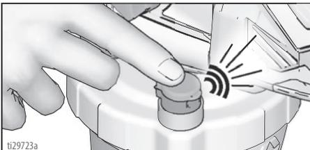
7. Install battery onto sprayer.
