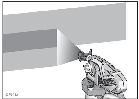
Rotating the spray tip guard changes the pattern to either the vertical or horizontal orientations.
