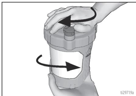
3. Align VacuValve on cup cover with Prime Pump/Spray knob. Push cup assembly onto sprayer and twist to lock.
