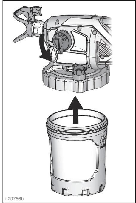
8. To clean the cup cover and pump filter shake the entire sprayer for ten seconds.
