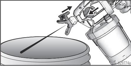
5. Turn Prime Pump/Spray knob down to Prime position. Rotate spray tip back to SPRAY position. Turn Prime Pump/Spray knob forward to SPRAY position, and resume spraying.
