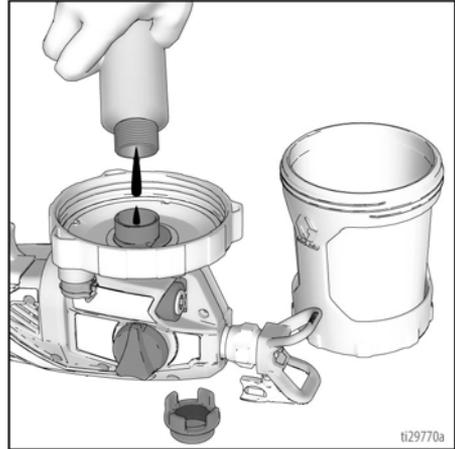
6. Install a clean pump filter into pump opening.
