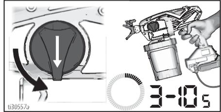
9. Air from pump may have entered the FlexLiner during priming. Repeat Steps 4 – 6 to ensure all air is evacuated.
