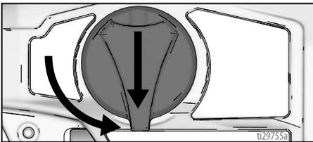
3. Separate the cup support with FlexLiner from the cup cover/sprayer. Set the sprayer upside down on a flat surface.
