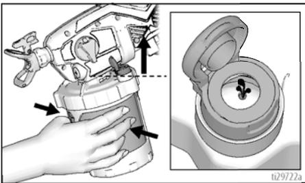
6. Stop squeezing the FlexLiner and snap the VacuValve cap closed. You will hear the cap click when it is closed properly.
