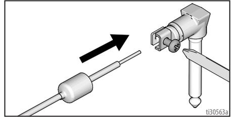
2. Loosen screw and remove broken wire. Insert stripped grounding wire and tighten screw.
