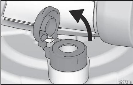
5. Open VacuValve cap. Tilt the sprayer so the VacuValve is the highest point, causing any air in the FlexLiner to rise to the VacuValve. Gently squeeze the FlexLiner to evacuate all air through the VacuValve air hole. Once you see material enter the VacuValve reservoir, all air should be evacuated from the FlexLiner.
