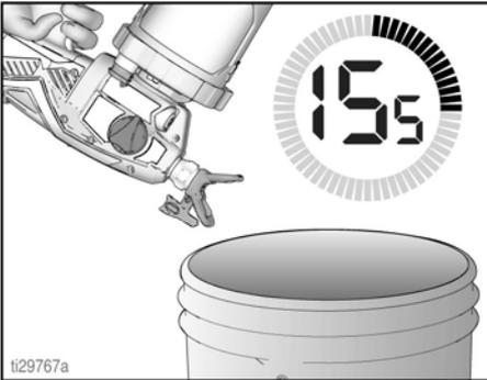
11. Turn Prime Pump/Spray knob forward to SPRAY position.
