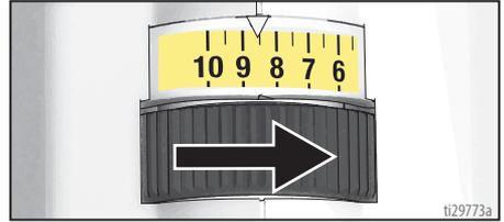
The speed control allows for infinite pressure adjustment. To reduce overspray, always start at lowest speed setting and increase speed to the minimum setting that results in an acceptable spray pattern.
