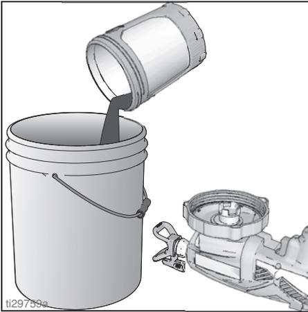
5. You can either dispose of the used FlexLiner and install a new FlexLiner or clean a used FlexLiner.
