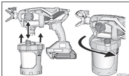
4. The VacuValve is an important part of your new sprayer. It is used to evacuate the air out of the FlexLiner. Sprayer will not spray if there is air in the FlexLiner.
