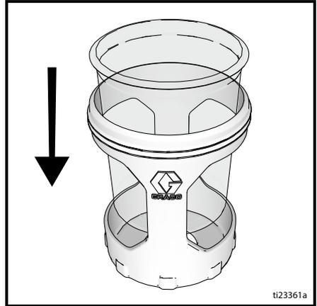
4. Fill FlexLiner with cleaning fluid. See **Cleaning Fluid Compatibility**, page 28.
