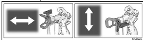
4. Hand tighten guard (25) retaining nut when you have adjusted to desired setting.
