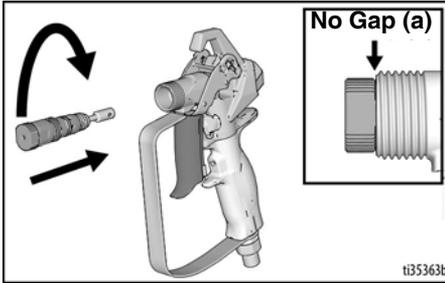
9. Push trigger assembly (13) back down into spray position. The push pins (11) should snap back out to normal position when trigger assembly (13) is fully engaged. Verify the cartridge is installed correctly by making sure the trigger assembly (13) can wiggle back and forth.
