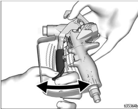
**NOTE:** Do not operate the gun if the cartridge is not installed correctly.
