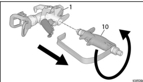
**Contractor PC Compact:** Unscrew handle (10) from housing (1) using guard (5).
