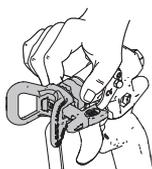
To prevent spray tip leaks make certain spray tip and tip guard are installed properly.
