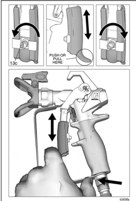
4. Tighten adjustment knob (13c) firmly.
