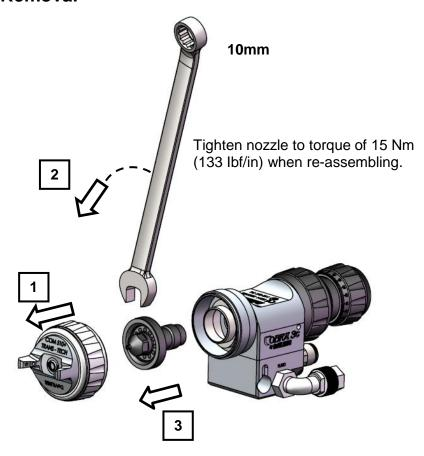
Manifold O-Ring and Connector Removal/Assembly
