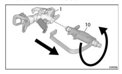
**Contractor PC Compact:** Unscrew handle (10) from housing (1) using guard (5).
