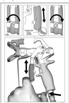
4. Tighten adjustment knob (13c) firmly.
