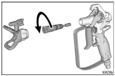
**NOTE:** If it is too difficult to remove by hand, use a 1/8" allen wrench or 5/8 wrench (if your cartridge has flats) to break loose as shown.
