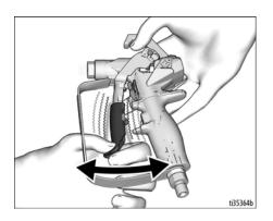
**NOTE:** Do not operate the gun if the cartridge is not installed correctly.
