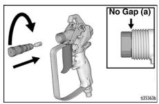
Push trigger assembly (13) back down into spray position. The push pins (11) should snap back out to normal position when trigger assembly (13) is fully engaged. Verify the cartridge is installed correctly by making sure the trigger assembly (13) can wiggle back and forth.
