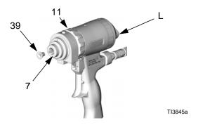
If mix module (39) does not protrude from fluid housing (7), slightly loosen then retighten lock ring (11), to allow gripping of edge for removal.
