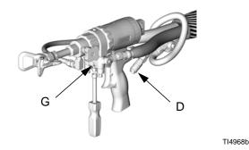
**4.** Unscrew cap (10) from stop (15), using two pair of channel-lock pliers. Inspect spring (17), safety actuator (3), bushing (4), and o-rings (14, 18).
