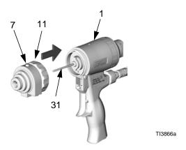
Push mix module (39) onto rod (31) as far as possible.
