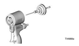
**9.** Install piston safety lock assembly until bottomed out.
