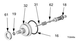
**8.** Liberally lubricate piston o-rings. Install spacer (61) onto piston assembly. Reinstall piston. Shaft is keyed for proper assembly. Push firmly to seat piston. Rotate piston/purge rod assembly clockwise with nut driver until piston is fully seated.
