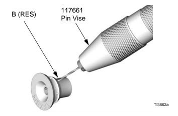
When drilling, be careful not to allow bit to come in contact with ID of mix module.
