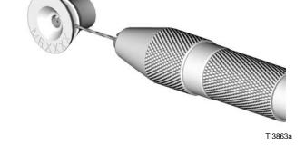
Fig. 1. Cleaning Component A (ISO) Ports
