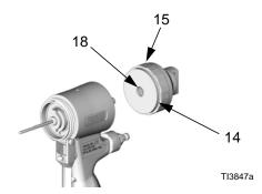
**6.** Pull purge rod to remove piston (32). Inspect piston o-ring (16) and shaft o-ring (19).
