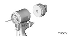
**9.** Reassemble the fluid housing onto the front end of the gun. See Reassemble Front End, page 32, steps 1 through 6.
