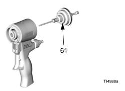
Spacer (61) is optional. For more forward travel of piston, remove spacer.
