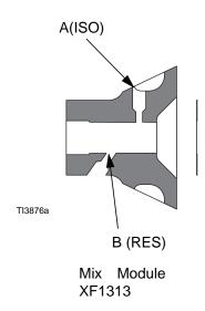
**5.** Open up resin porting to raise ISO pressure. Starting with the smallest drill bit size, drill into port. For drill bit sizes, see **Drill Bit Table**, page 16.
