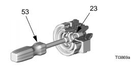
**6** Push out rear seal (46) with screwdriver (54).
