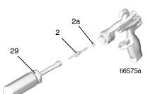
leaking, replace the entire needle assembly. If replacement is necessary, be sure to remove the o-ring (2a) as it may stick inside the gun body.
