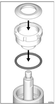
11. Install pump rod adapter, torque to  $35 \pm 5$  ft-lbs (47 ± 7 N•m)
