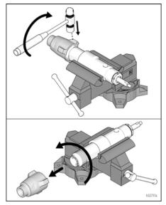
3. Loosen and remove packing nut.
