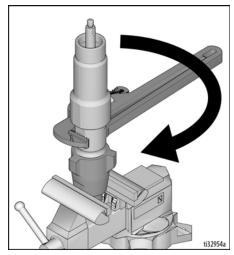
Install O-ring and Packing Nut. Torque packing nut to 25 ± 5 ft-lbs (34 ± 7 N•m).
