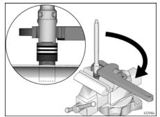
4. Assemble throat packings and place in pump cylinder.
