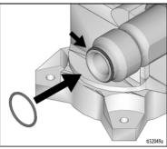
8. Clean seat thoroughly. Reassemble intake valve with a seat, ball, and new o-ring. Seat may be flipped over and used on other side.
