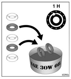
2. Assemble packings and ball to piston and piston rod.
