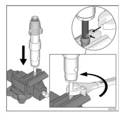
2. Unscrew cylinder from intake valve.
