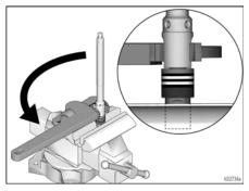
6. Remove piston from displacement rod. Clean and inspect parts.
