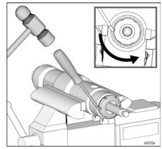
Tap piston rod out of cylinder with a plastic hammer being careful of the threads. Use a thin, soft rod if necessary.
