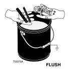
5. Attach ground wire to true earth ground or plug unit into grounded outlet.
