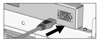
When power is connected the voltmeter will turn on and the charger will immediately begin charging.
