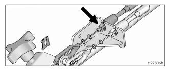
Install cable end onto trigger plate pin and install clip.
