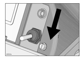
3. Turn prime valve down. Turn pressure control counterclockwise to lowest pressure.
