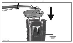
11. Trigger all guns again into a flushing fluid pail until paint appears. Assemble tips and guards.
