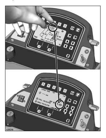
4. Press B to transfer calculated dot spacing distance to Layout Mode. Save this value in favorites if desired.
