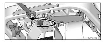
2. If striper arcs to the right, loosen left set screw and tighten right set screw for fine tune adjustment.
