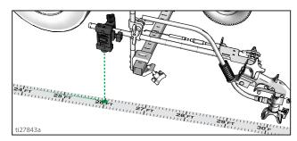
Press and release gun trigger control to complete calibration.
