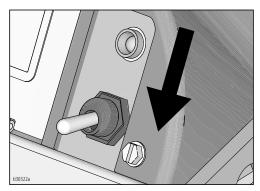
Plug charging cord into charging port on the unit. Connect an extension cord, minimum 12AWG (2.5mm²), to the charging cord and plug it into wall power.
