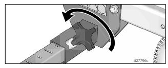
2. Slide gun arm assembly (including gun and hoses) out from gun arm mounting slot.
