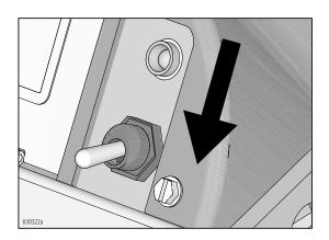
3. Turn pressure control to lowest setting. Trigger all guns to relieve pressure.
