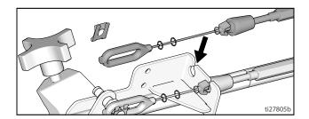
3. Insert plastic cable retainer into cable bracket hole.
