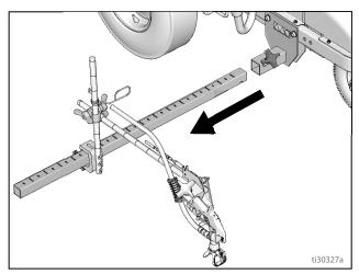
3. Slide gun arm assembly into desired gun arm mounting slot.
