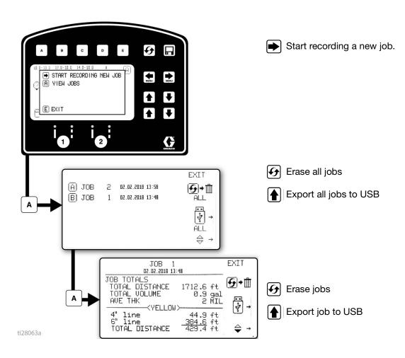
Job data is compiled while spraying. A summary of volume sprayed, distance sprayed and average mil thickness is displayed for the entire job. The job is also broken down by colors, line widths and stencil volume sprayed.
