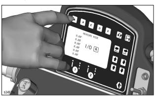
3. Press and release **A** to end measured length. Up to six lengths are viewable.
