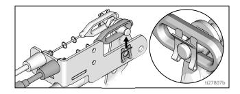
Route cable around unit and up through cable holes behind hose mount.
