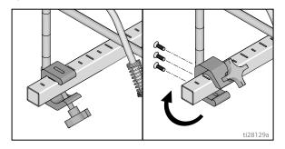
Another option can be to swing the gun out at an angle and rotate the tip guard. This results in better visibility for the user.
