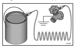
To maintain ground continuity when sprayer is flushed or pressure is relieved: hold metal part of spray gun firmly to the side of a grounded metal pail then trigger the gun.
