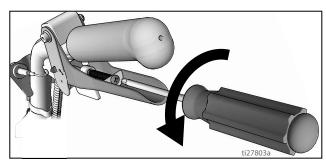
Continue adjusting screw in handle until timing of spray icon and fluid spray are synchronized.
