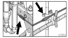
1. Use wrench to loosen locking nut on cable adjuster.
