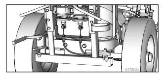
Route cable end loop through rectangular hole in bracket and insert plastic cable retainer into the actuator bracket. Install cable end onto actuator rod and install pin.
