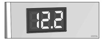
Battery will charge to 14.6-14.8 volts and then it will come back down to ~13.6 volts when fully charged.
