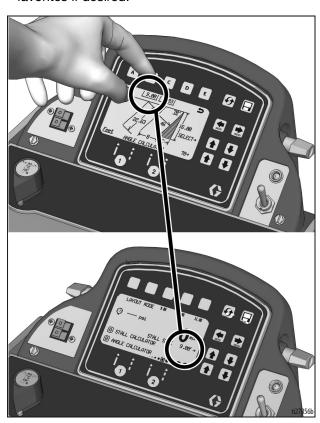
5. Press and release gun trigger control to start marking stall size dots. Press and release gun trigger control to stop marking.
