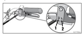
a. One gun: Disconnect one gun selector plate from trigger.
