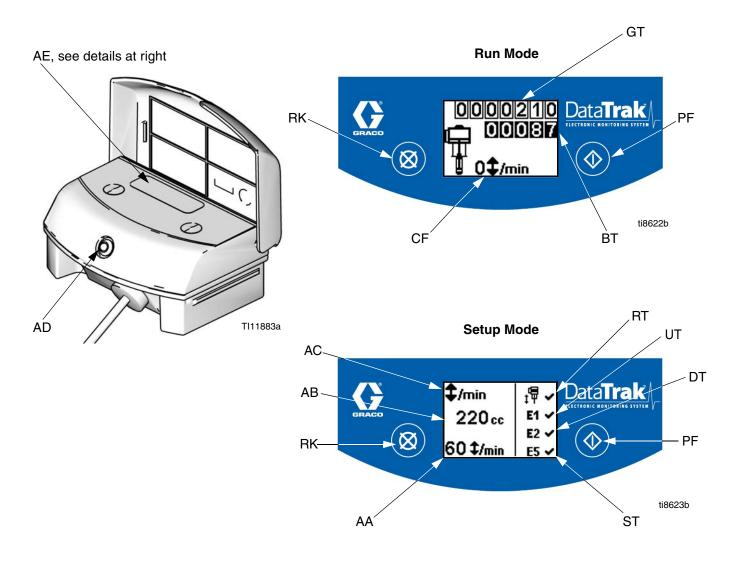
Fig. 7. DataTrak Controls and Indicators
