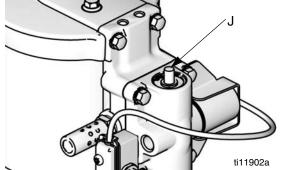
Fig. 8. Solenoid Release Button
