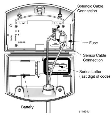
Fig. 11. DataTrak Battery and Fuse Location
