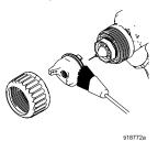
7. If necessary, use a toothpick or other soft tool to clean the air cap holes. Do not use metal tools.
