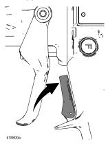
6. Trigger the gun into a grounded metal waste container to relieve the fluid pressure.
