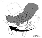
5. Disengage the trigger lock.
