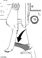
8. Open the pump drain valve, having a waste container ready to catch the drainage. Leave the pump drain valve open until you are ready to spray again.
