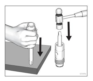
5. Unscrew piston valve from piston rod. Clean and inspect parts. The piston has a special thread locking/sealing patch. Do not remove the patch. The patch allows four disassembly/assembly procedures before it is necessary to apply medium strength threadlocker to the threads.
