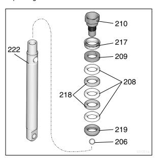
2. Install ball (206) in piston rod. If threadlocker is applied to piston valve threads, make sure that none gets on ball.
