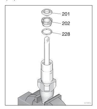
2. Unscrew intake valve from cylinder.
