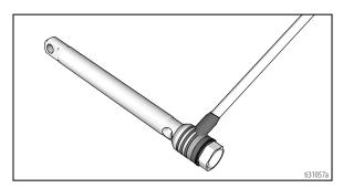
7. Grease top inch or two of piston rod that will go through the cylinder throat packings.
