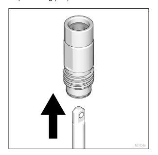
9. Reassemble intake valve with new o-ring (227), seat (212) and ball (214). Seat may be flipped over and used on other side. Clean seat thoroughly.
