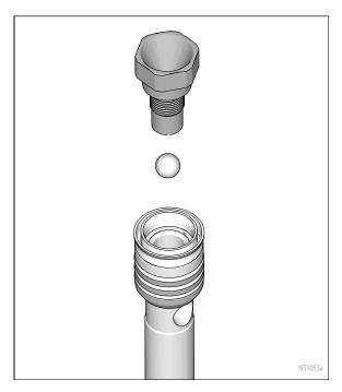
3. Tighten piston valve to piston rod. torque piston valve to  $27 \pm 3$  ft-lb.  $(37 \pm 4.1 \text{ N} \cdot \text{m})$ .
