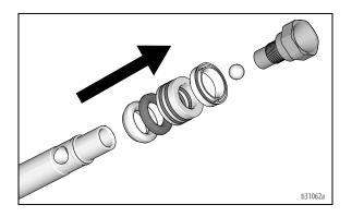
7. Remove throat packings and glands from cylinder. Discard throat packings and glands.
