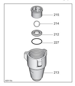
10. Install intake valve on cylinder. If a wrench is used torque to  $60 \pm 5$  ft-lb  $(81 \pm 7 \text{ N} \cdot \text{m})$ .
