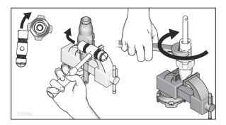
Disassemble intake valve. Clean and inspect o-ring (227). NOTE: A pick may be required to remove o-ring.
