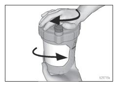
3. Align VacuValve on cup cover with Prime Pump/Spray knob. Push cup assembly onto sprayer and twist to lock.
