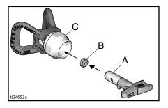
3. Insert Spray Tip. Spray tip must be pushed all the way into the tip guard.
