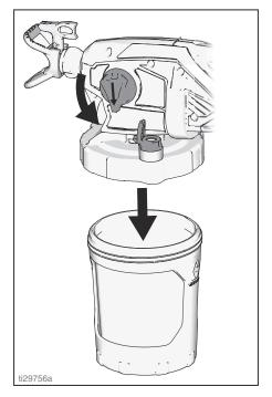
3. Set the sprayer upside down on a flat surface. This will keep the wet paint in the cup cover. Return excess material to original container. Hold the FlexLiner in place when pouring.
