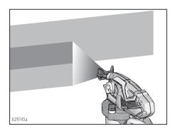
Rotating the spray tip guard changes the pattern to either the vertical or horizontal orientations.
