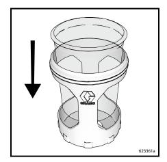
4. Fill FlexLiner with cleaning fluid. See **Cleaning Fluid Compatibility**, page 27.
