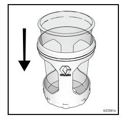
2. Fill FlexLiner with material. Securely tighten cup cover onto cup support. For proper sprayer operation lid must seal tightly with the cup.
