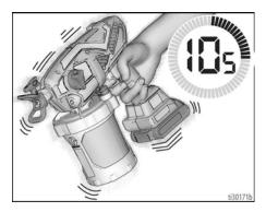
8. Make certain the Prime Pump/Spray knob is in the Prime Pump position (pointed down). Set speed control to 10.
