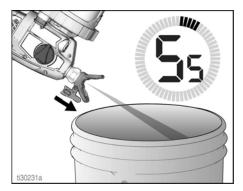
b. Reverse the spray tip to UNCLOG position, pull the trigger for five seconds. Release the trigger.
