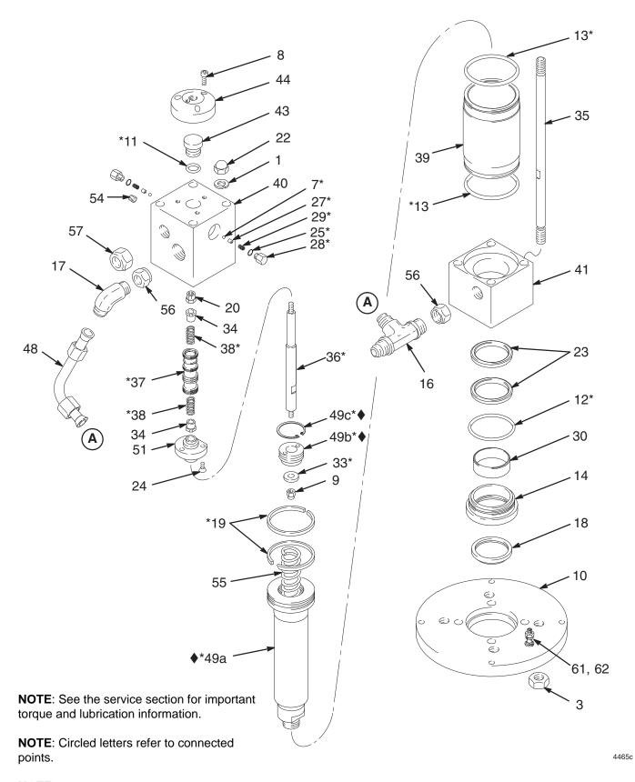
**NOTE**: Graco recommends replacing 49a, 49b, and 49c all together in Kit 26C141.
