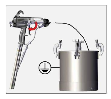
4. Load next color, solvent flush and/or remove applicator from installation as required.
