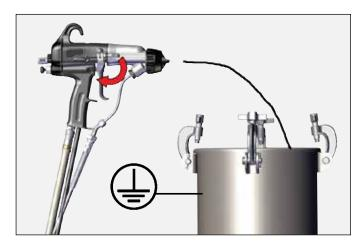
4. Release trigger stop material flow.
