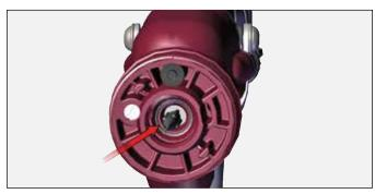
3. Install fluid nozzle using 80353-00 wrench. Tighten till nozzle seats on O-ring and then 1/8 additional turn.
