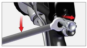
3. Remove rear cover and cartridge with 15mm wrench.
