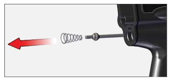
4. Remove air valve packing nut and packing.
