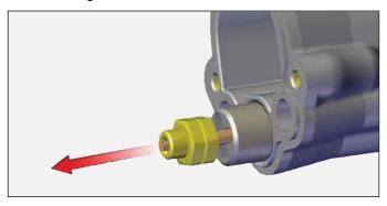
4. Remove jam nuts using 10mm wrench.
