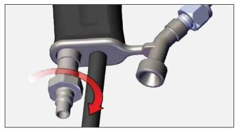
3. Remove bracket, gasket and o-ring.
