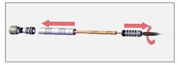
6. Prior to installation apply dielectric grease inside packing tube, completely full.
