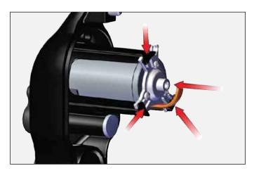
3. Install cartridge then o-ring (if removed).
