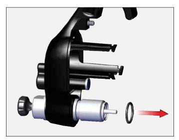
6. Push on edges to remove fluid valve cartridge.
