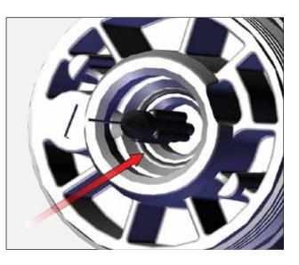
3. Install fluid nozzle using 80353-00 wrench. Tighten till nozzle seats on O-ring and then 1/8 additional turn.
