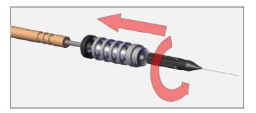
8. Insert packing tube onto shaft. Wipe excess grease over front parts and outside of packing tube.
