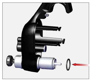
4. Install screw and retainer.
