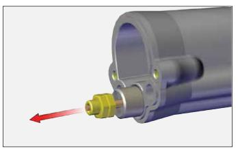
4. Remove jam nuts using 10mm wrench.
