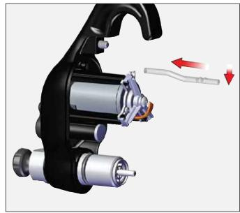
6. Install fluid valve cartridge.
