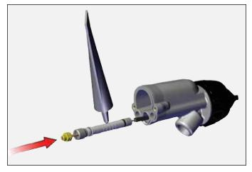
2. Tighten packing using wrench. Pull back and forth on the needle shaft till a slight amount of drag is felt.
