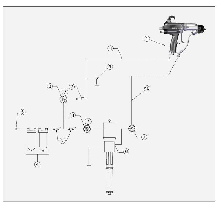
Figure 2: Ransflex Typical Solventborne Installation
