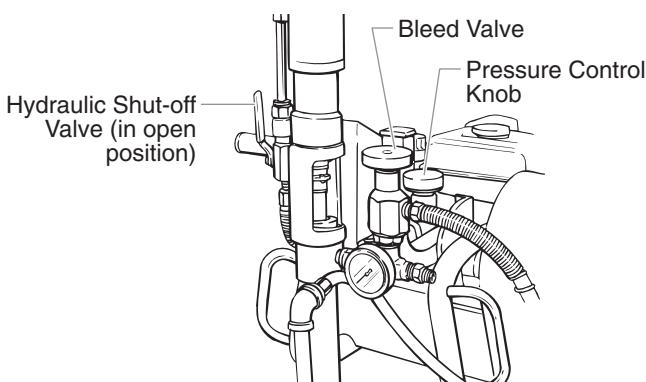
5. Open the hydraulic shut-off valve located on the hydraulic pressure hose. The handle should be in line with the hose.
