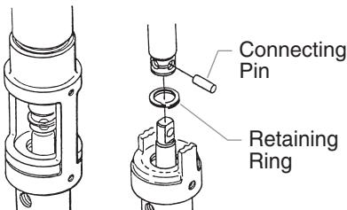
9. Remove the piston rod assembly from the motor/pump block (31).
