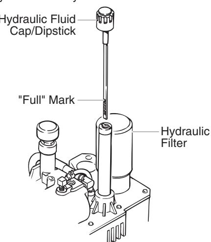
**NOTE: When replacing the hydraulic filter during a fluid change, it may be necessary to add up to one additional quart of hydraulic fluid.**
