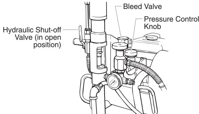
6. Open the hydraulic shut-off valve located on the hydraulic pressure hose. The handle should be in line with the hose.
