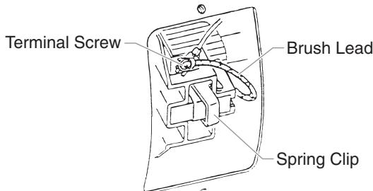
3. Loosen the terminal screw. Pull the brush lead away, but leave the motor lead in place. Remove the brush and spring.
