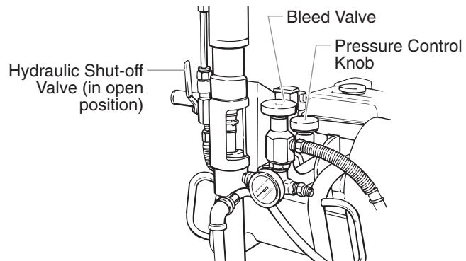
4. Open the hydraulic shut-off valve located on the hydraulic pressure hose. The handle should be in line with the hose.
