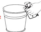
13. Trigger the gun into the metal waste container until the paint is flushed out of the hose and solvent is coming out of the gun.
