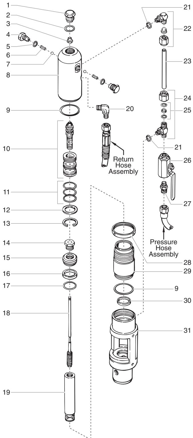
**NOTE:** Refer to the "SAE O-Ring Fitting Installation" procedure at the end of this section for installation instructions for item 22.
