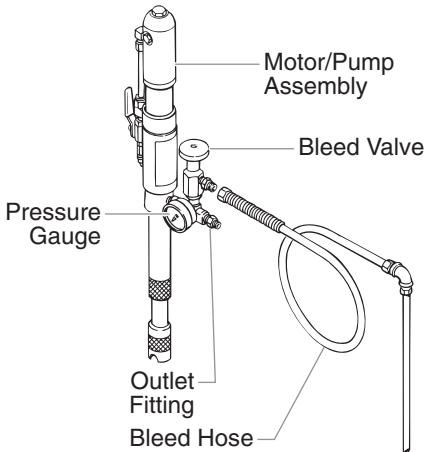
2. Attach a minimum of 50' of nylon airless spray hose to the outlet fitting. Do not use Teflon tape or thread sealant on the spray hose connection.
