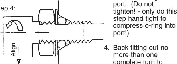
3. Screw fitting in until washer pushes o-ring into entrance and sits flat against port. (Do not tighten! - only do this step hand tight to compress o-ring into port!)
