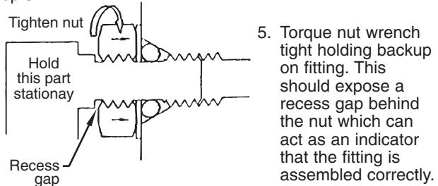
5. Torque nut wrench tight holding backup on fitting. This should expose a recess gap behind the nut which can act as an indicator that the fitting is assembled correctly. (This is a feature for a specific version of this fitting only - which screws into the cylinder head.)
