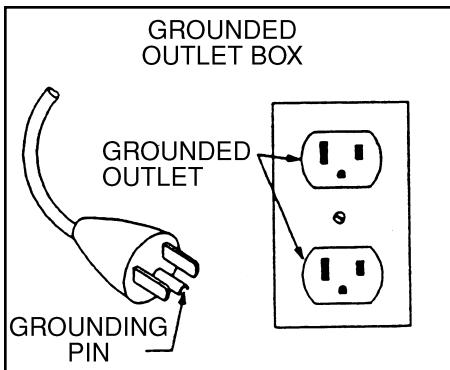
wire for the electric current. This product is equipped with a cord having a grounding wire with an appropriate grounding plug. The plug must be plugged into an outlet that is properly installed and grounded in accordance with all local codes and ordinances.
