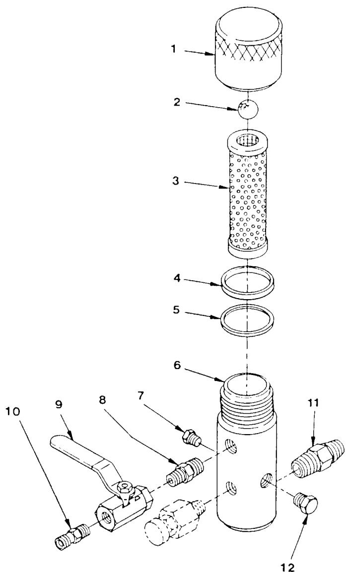
OUTLET MANIFOLD FILTER ASSEMBLY PART NO. 920-560
