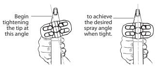
9) Insert spray tip (tip pointing in the spray direction).
