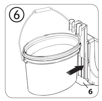
• Push the height-adjustable paint bucket attachment (fig. 7, 5) down in order to secure the bucket.
