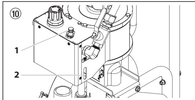
Check the injection rate by observing the flow through the openings in the side of the air motor shroud.
