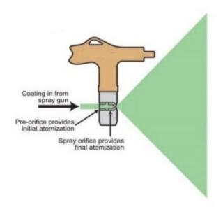
The finer atomization of the spray allows much lower application pressure. Traditional airless spray tips require approx 2000psi to produce the correct spray fan without leaving "tram line" or "tracks" at the top and bottom of the spray fan but the Atomex X-50CT will perform and give you a great spray finish at pressures as low as 1300psi (depending on the product applied)
