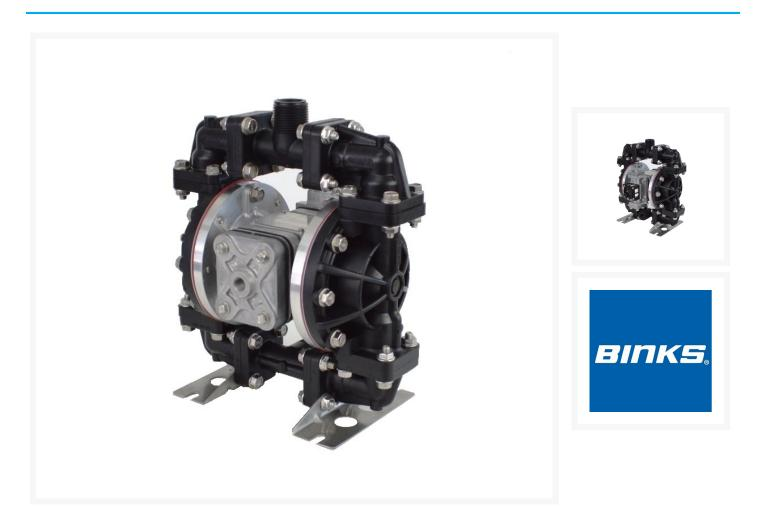
Binks 41-818831 1/2" Acetal Short Stroke Double diaphragm pump features PTFE Diaphragms, 316 Stainless Steel Balls & Check Valve Seats. Short stroke pump has an optimized diaphragm design and reduction in stroke length to provide efficient pump changeover and is ideal for low pressure spraying applications.
