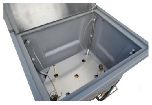
The unit can clean two guns at once, simply fit the trigger clip onto the gun to keep the trigger open, invert the gun over the vertical washer jet, thinners will be pumped through the gun and a fine mist of thinners will be sprayed on the outside of your gun washing away any paint on the outside of the gun.
