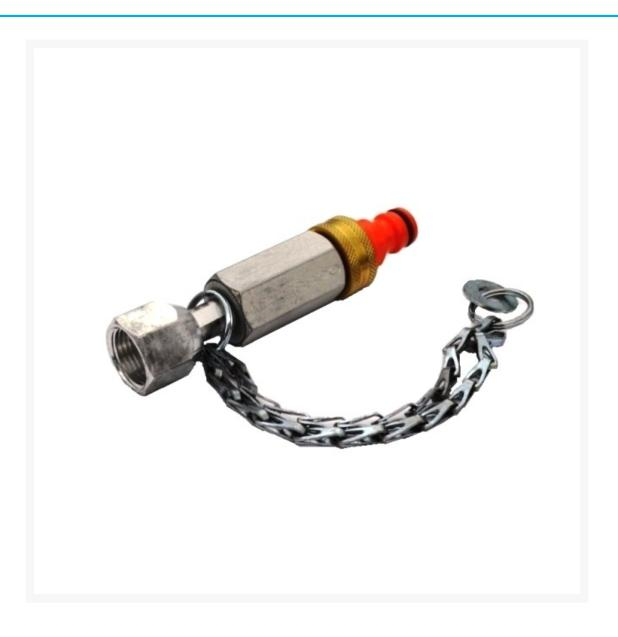
Airlessco 170-005 Quick Flush System allows the user to flush water-based paints back through the gun and hose into the original paint container. It fits between an airless gun and a garden hose, and it cuts typical clean-up time in half.
