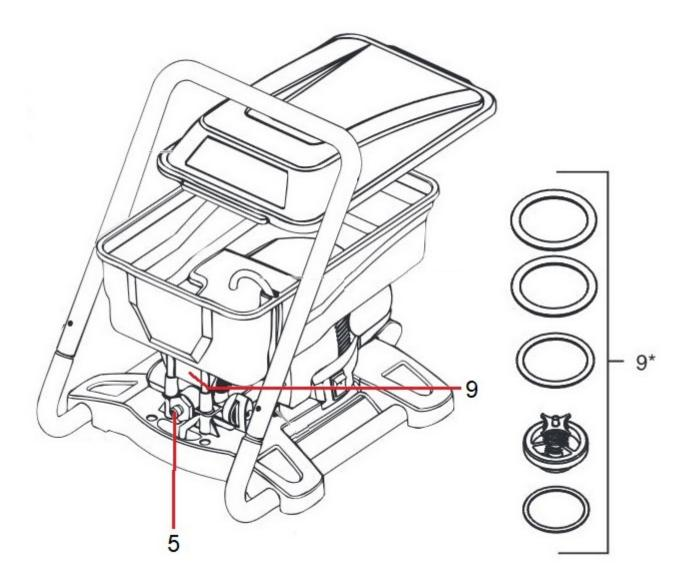
Wagner 0515221 Paint Crew Inlet Valve Repair Kit is used with the following models -
