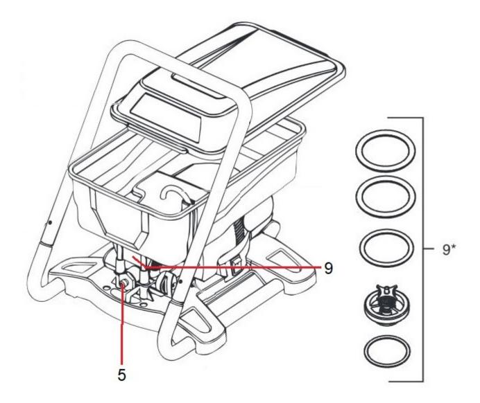
Wagner 0515237 Paint Crew Outlet Valve Repair Kit is used with the following models -
