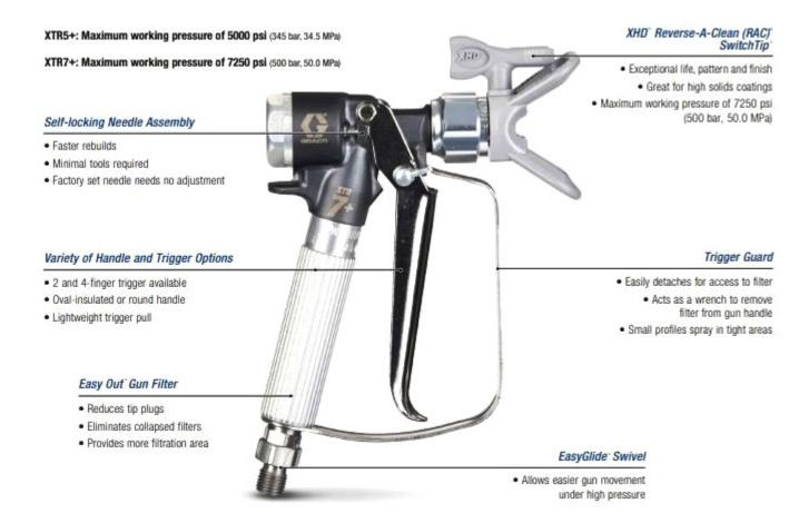
Graco XTR724 Heavy Duty Airless Spray Gun is standard with Round Handle, 4-Finger Trigger, XHD RAC Tip.
