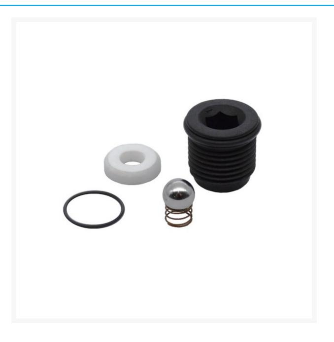
Wagner 2399783 Control Pro 150 Inlet Valve Kit is required when servicing your Control Pro 150. Worn inlet valves should be replaced if your sprayer will not hold pressure.
