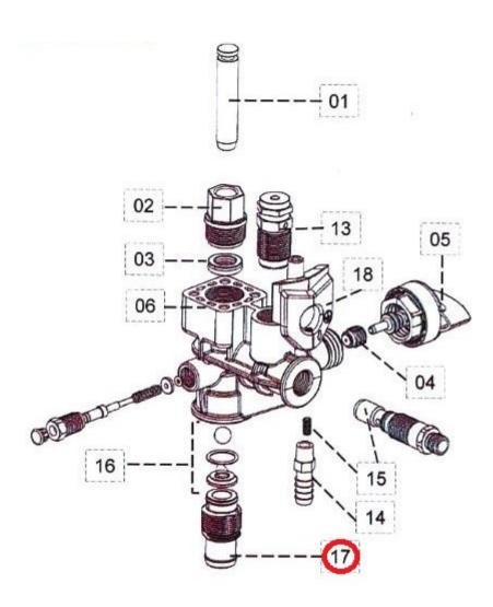
Wagner 0580071A Control Pro 250/350 Inlet Valve Housing is used with the following models -
