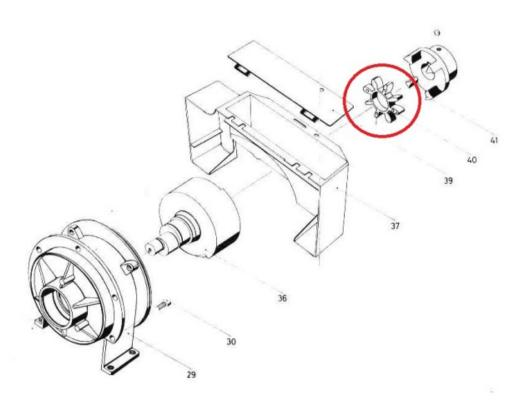
Wagner 9993806 Gear Rim allows safe power transmission by absorbing peak loads and torsional vibrations. Moreover, the elastic design of the polyurethane gear rim compensates for angular and radial misalignments and also absorbs small shaft length variation.
