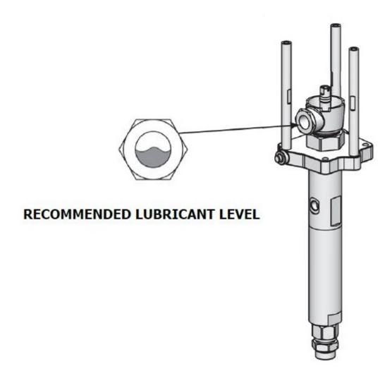
Binks Pump Lube is available in solvent based 0114-016099
