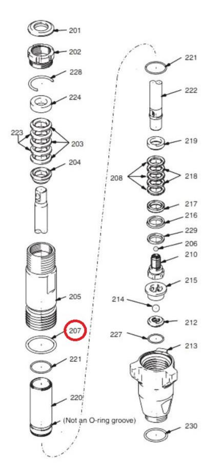
People commonly replace this o-ring when they have a leak at the foot valve but this o-ring will not fix this problem. You should consider replacing the 106526 packing o-ring which is located at the end of the pump sleeve and consult the user manual for your machine.
