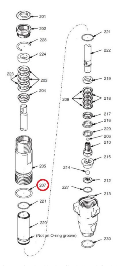
People commonly replace this o-ring when they have a leak at the foot valve but this o-ring will not fix this problem. You should consider replacing the 107098 packing o-ring which is located at the end of the pump sleeve and consult the user manual for your machine.
