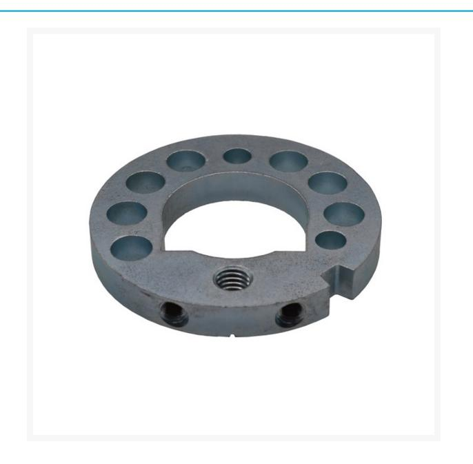
Graco 17H486 Disk Adjuster Assembly is used throughout the range of LineLazer IV & V Series machines. The disk adjuster is located between the fork and the castor assembly and allows alignment/adjust of the front wheel.
